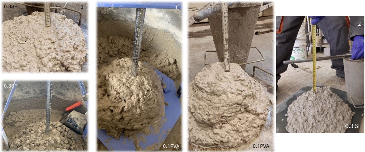
Fig. 3 Slump test performed by participants 1, 2, and 3
