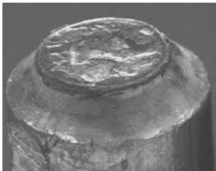
Fig : Example of electrode with heavy wear.
