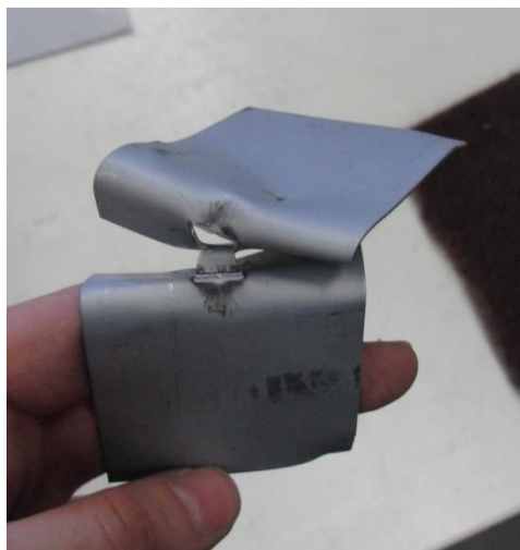
Figure 16.11: Peel test of the steel (left) and aluminum samples (right).
