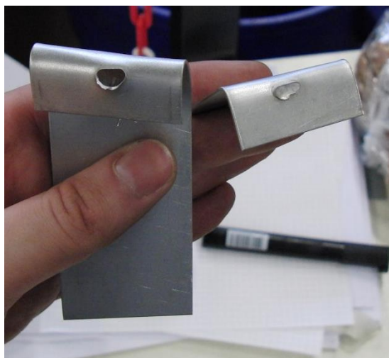
Figure 16.11: Peel test of the steel (left) and aluminum samples (right).
