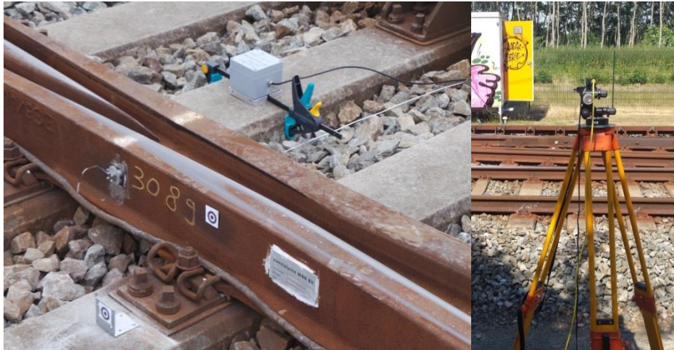
Figure 2.1 Instrumented frog with ESAH-M sensors and Video Gauge targets/camera
