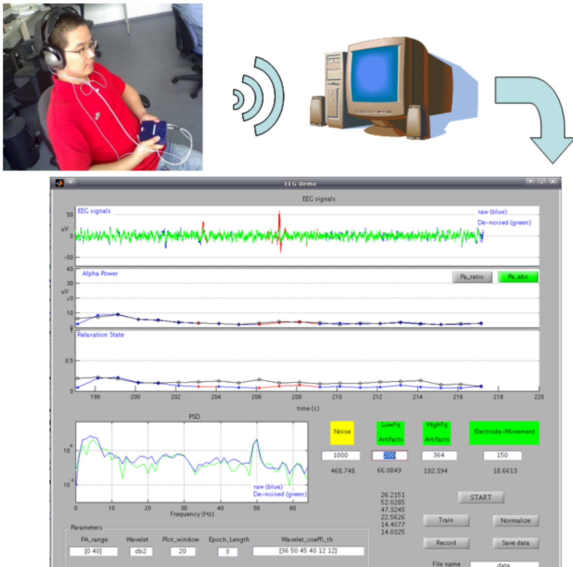
Figure 5-4: The realization of real time alpha wave measurement. Top left: subject with EEG measuring headphone and nexus. Bottom: Graphical User Interface to monitoring and recording EEG signals.
