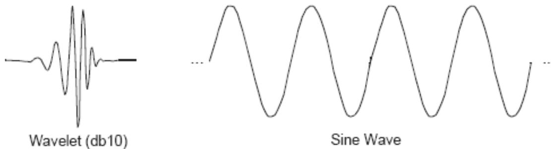
Figure 3-1: Comparison of wavelet and sine wave. Sinusoids are smooth and predictable. Wavelets are irregular and asymmetric.
