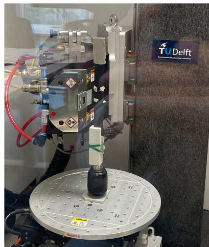
Figure 4.13: Specimen inside the micro-CT scanner. Scanned regions are marked with strips of tape that indicate the desired alignment of the X-ray cathode.
