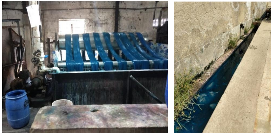
Figure 4.8: Dyeing process in action in an industry in Badai (L). Waste water discharged from the industry (R)
