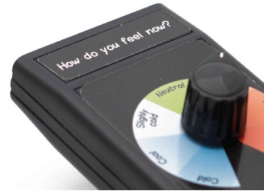
Fig. 2. Comfort Dial used to capture perceived comfort levels of tenants during the Ecommon measurement campaign.
