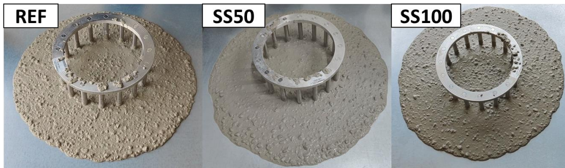
Fig. 4 J-ring slump-flow of SCC mixtures
