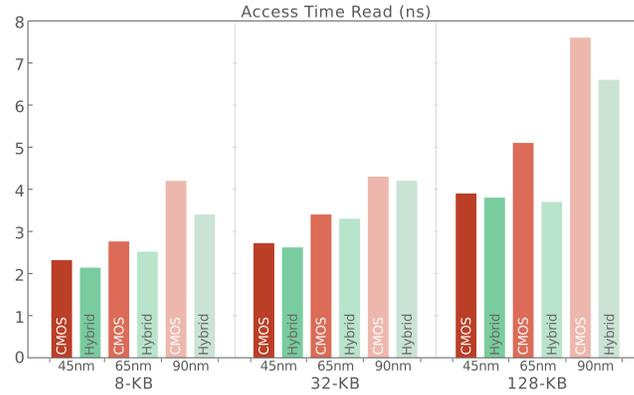
**Figure 7.16:** 64-bit Word Width Memories Read Access Time
