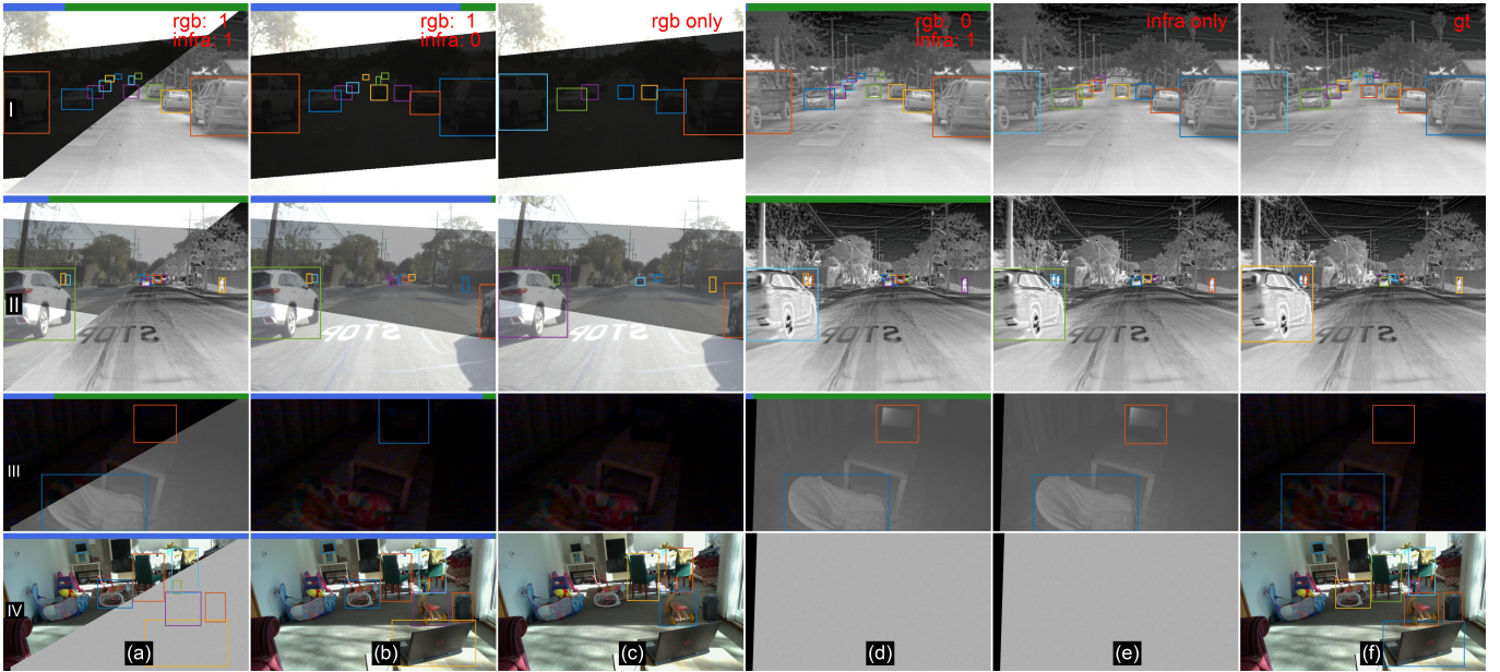
Fig. 5. Qualitative analysis of our multi-modal object detector, g_{sa} in this case. Columns (a), (b) and (d) are the outputs of g_{sa} in various asymmetric sensor failure conditions imitated artificially, which are mentioned on the upper-right corner of each image in row I. The top blue/green bar represents the contribution of each sensor modality in obtaining the final results (RGB: blue and Thermal/Infra: green). (c) and (e) are the outputs from single modal baselines. (f) is the ground-truth. Rows I and II are from FLIR-Thermal dataset while III and IV are from L515-Indoor dataset. Row IV represents a true sensor failure case when IR camera gets saturated due to sun-light even in indoors.
