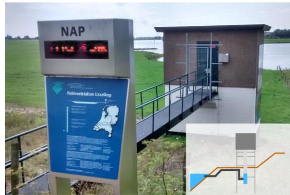
Figure A-3: The water level monitoring station for the IJsselkop. In the lower-right corner a cross-section of the measuring method with a monitoring well
