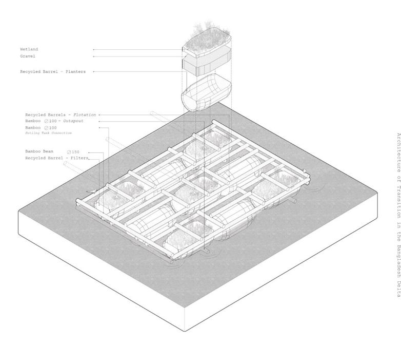
During the monsoon season, the raft rises with the rising water levelsalongside the helophyte filter. This adaptive system ensures that treated water is safely discharged into the surrounding environment
