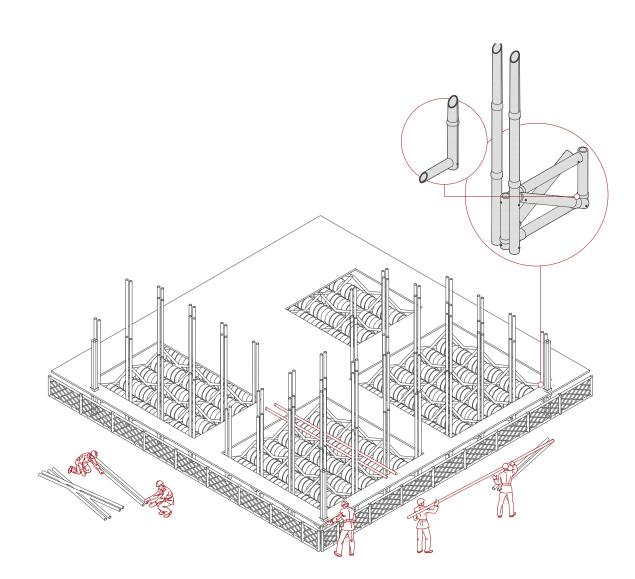
The vertical structural elements of the dwelling are bolted with the rafts cross bracing to ensure the stability of the project
