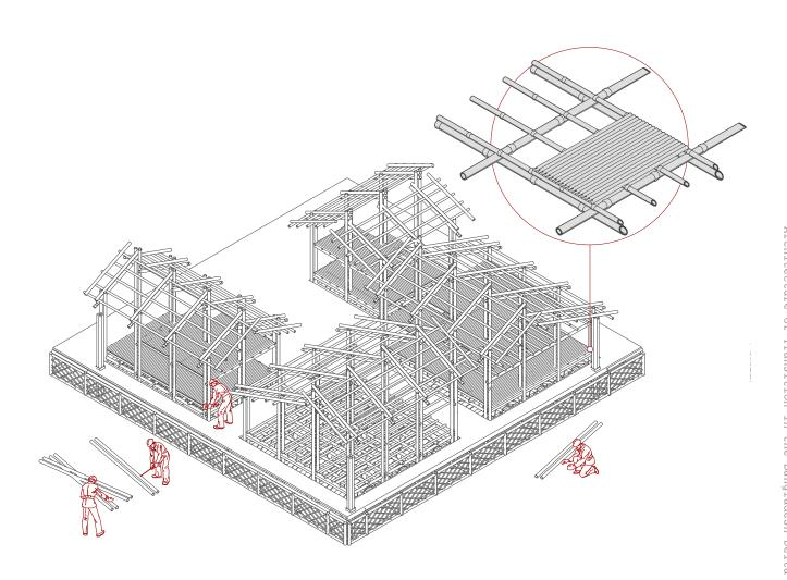
The split bamboo flooring is placed perpendicular to the horizontal structural elements and bolted into place
