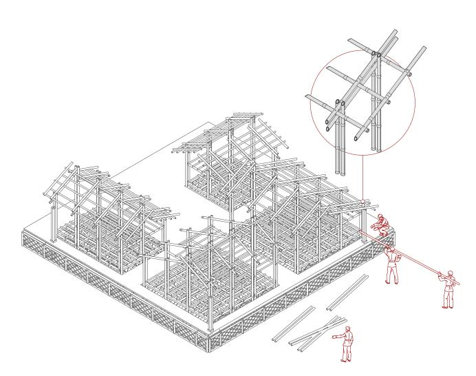
The roof elements are interlocked and bolted with the vertical structural elements
