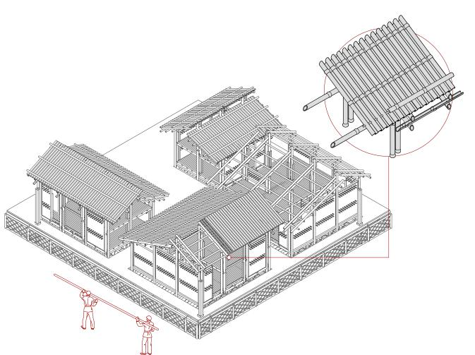
The split bamboo roof is designed with water collection in mind. A bamboo element runs through the culms and above to secure them in place
