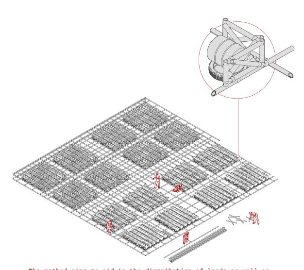
The method aims to aid in the distribution of loads as well as resist forces from different directions
