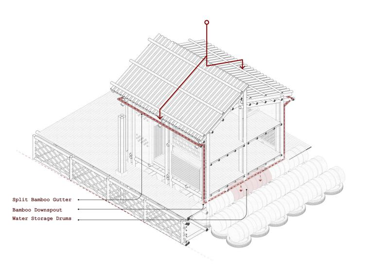
Three drums, with a total capacity of 630 liters, are installed within the dwelling to function as a ballast system. This arrangement ensures that the household maintains an adequate water supply for approximately one week.
