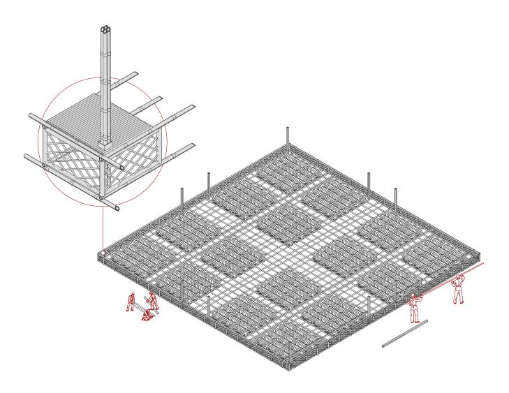
Four bamboo culms are bolted together to increase the lateral strength during flash flooding
