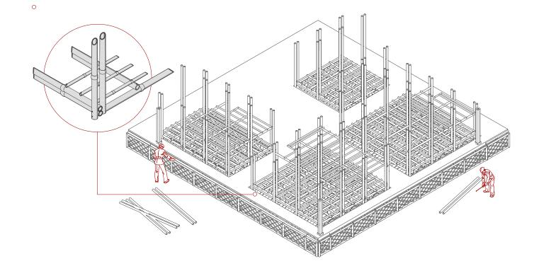
The horizontal structural elements are interlocked and bolted with the vertical structural elements
