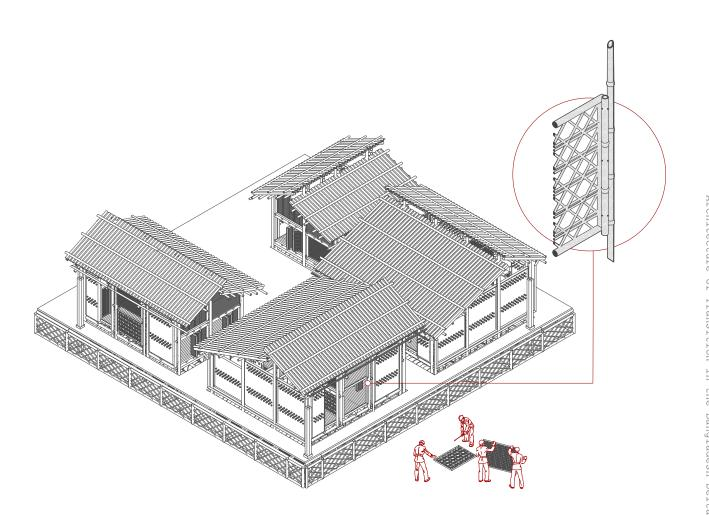
A series of bamboo panels have been designed to serve a series of functions within each dwelling
