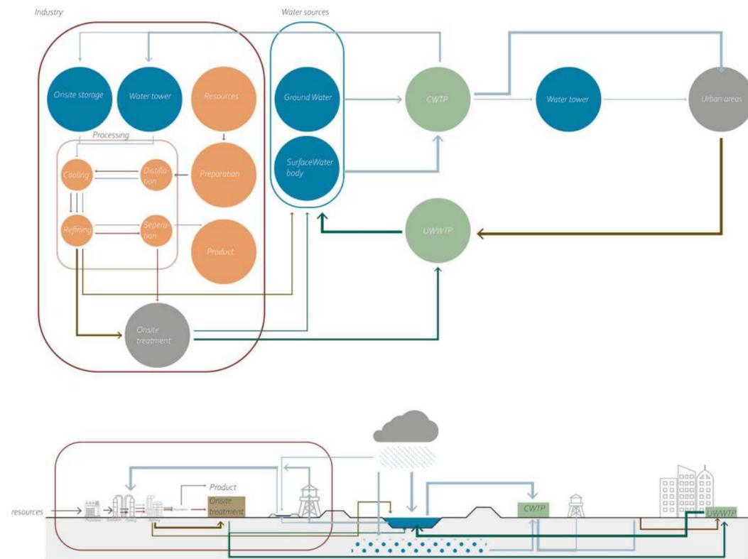
Figure 3.7 Current state of the industrial water system in diagramme and section.
