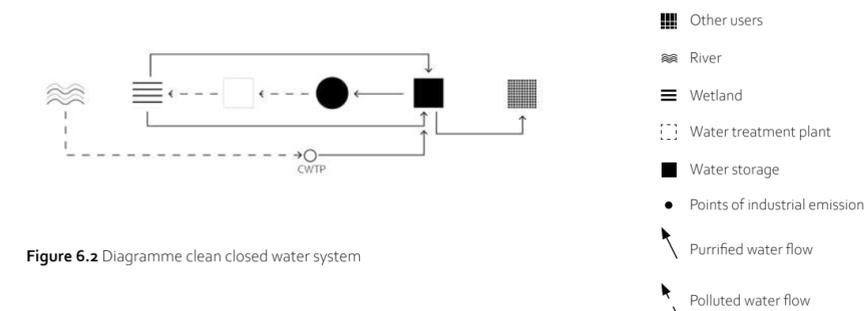
Figure 6.2 Diagramme clean closed water system
