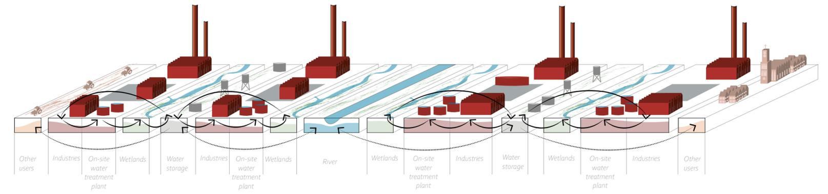
Figure 6.5 Decentralized closed loops with collective water storage
