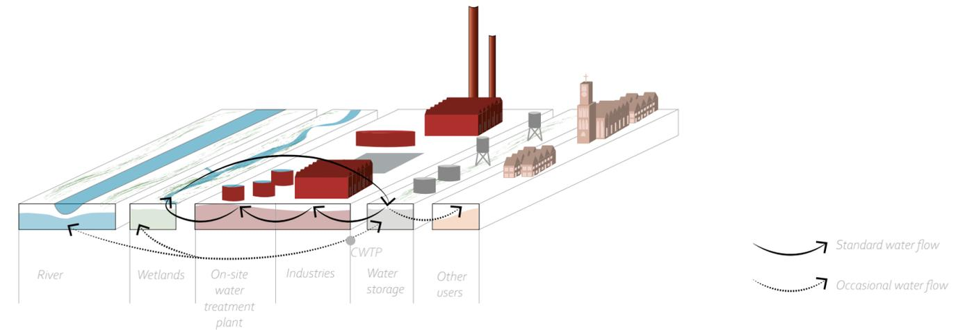
Figure 6.1 Clean closed water system
