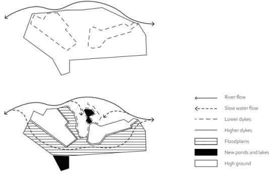
Figure 7.4 Gat van Den Ham flooding prevention system
