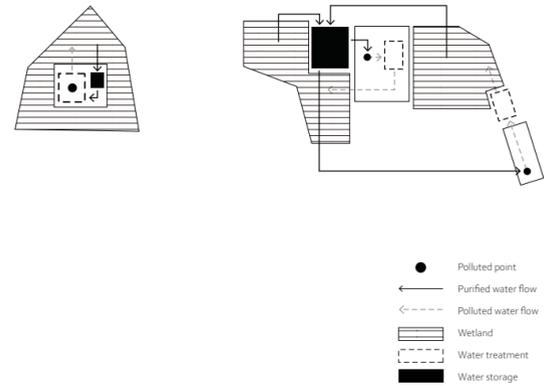
**Figure 7.5** Geertruidenberg distant closed loop system and local closed loops system
