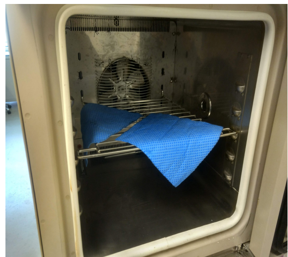
Figure 9. Placement of PVA inside the chamber
