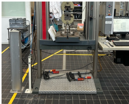
Figure 4 Universal Testing Machine Zwick Z100 with a maximum load of 100kN
