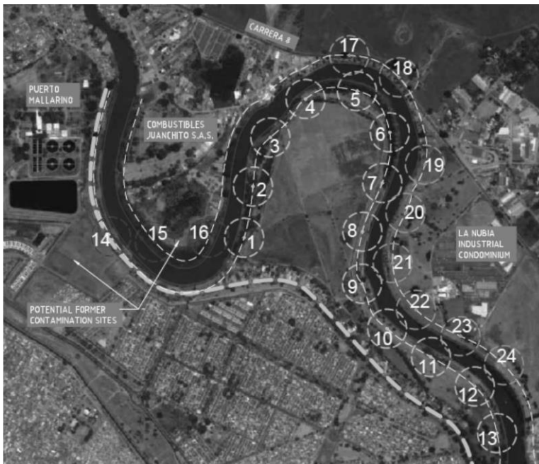
Figure 8. Scheme of potential locations to study RBF near the Puerto Mallarino WTP
