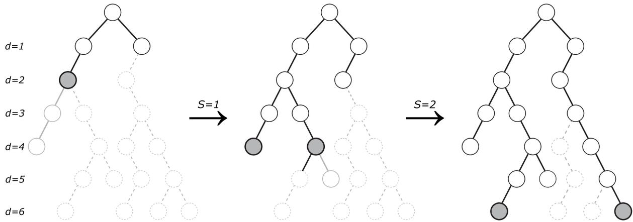
Fig. 4. OASP search tree with  $M = 2$  discrete actions,  $S = 0$  initial value and increment rule:  $S \leftarrow S + 1$  if the deepest expanded node is at  $d = (S + 1) \cdot 2$ . Nodes not yet expanded are marked in gray outline, nodes not eligible for expansion are marked with dashed line, whereas nodes filled with gray are those where the increment rule can be activated. All the nodes have 2 children, although the figure does not show all of them to limit the focus to the expanded nodes.
