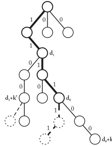
Fig. 3. OSP search tree with  $M = 3$  different actions,  $S = 3$  switches allowed and a single optimal path, marked with bold. Rewards are marked on the transitions. All the rewards outside the optimal path are zero. Dashed circles indicate nodes not belonging to the OSP tree. Note that some leaf nodes are not represented to reduce the complexity of the figure.
