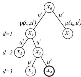
Fig. 1. OPD search tree with states in the nodes and actions and rewards on the arcs (corresponding to transitions). The size of the action space is  $M = 2$ . Note that some states may appear several times in the tree as results of different action sequences. The algorithm does not exploit these duplicates, but keeps them separate on the tree.
