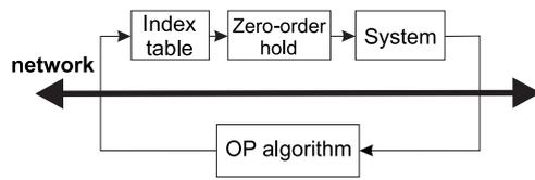
Fig. 7. Networked control system architecture.
