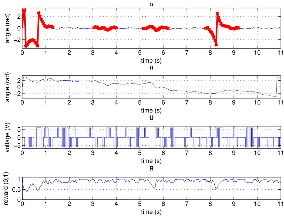
Fig. 9. Rotational pendulum online trajectory: the graphs show, from top to bottom, the evolution of the angular position of the pendulum ( $\alpha$ ) and of the actuated joint ( $\theta$ ), the control inputs  $U$ , and the rewards.
