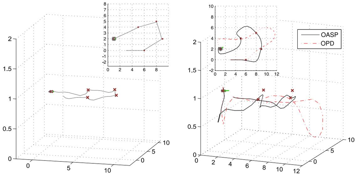
Fig. 12. Quadrotor online simulations: path obtained with LQR (left) and with OPD and OASP (right). Both figures show the flights in side view, while the insets show the trajectory in top view.
