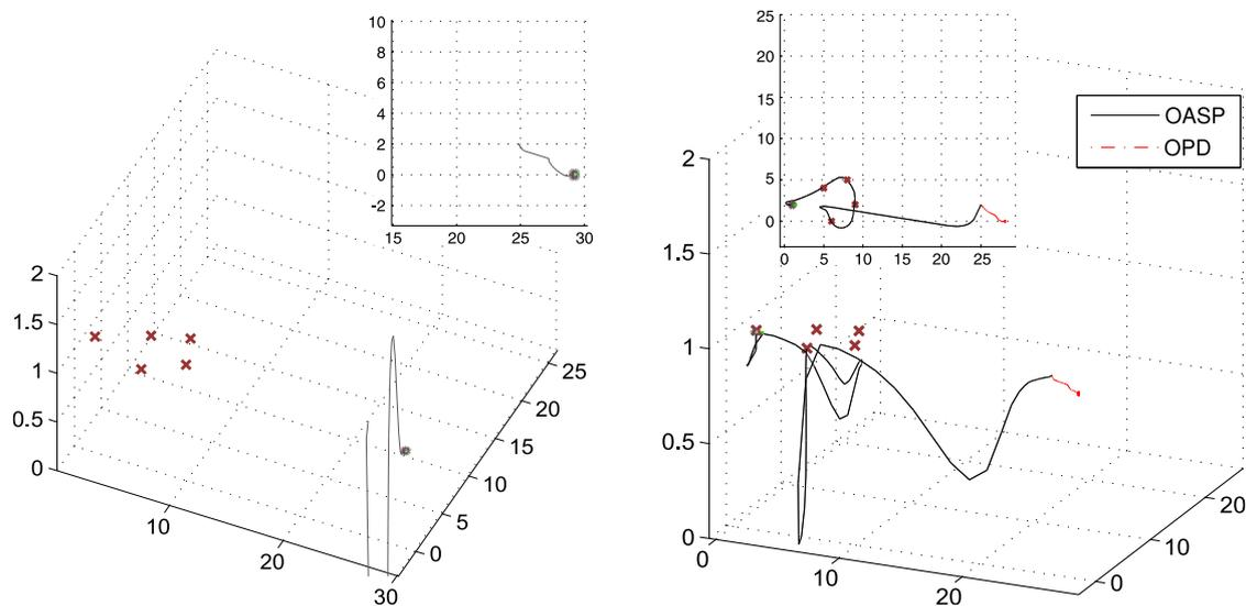
Fig. 13. Quadrotor online simulations: path planned with LQR (left) and with OPD and OASP (right).
