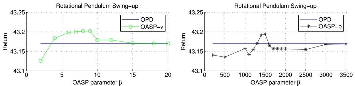
Fig. 11. Rotational pendulum: given a fixed computational budget of  $n = 1000$  expansions, the left graph shows the return obtained by OASP- $v$  for  $\beta \in [2, 20]$ , while the right graph presents the returns of OASP- $b$  for  $\beta \in [200, 3500]$ . Both graphs present as a reference the return obtained by OPD with  $n = 1000$ .
