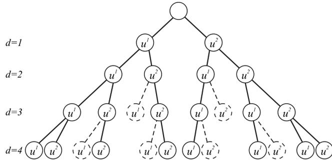
Fig. 2. Uniform expansion of the OSP search tree, with  $M = 2$  different actions and  $S = 1$  switch allowed. The action leading to a node is put in the node. Nodes preceded by continuous lines are expanded with all  $M$  actions. Nodes on the dashed paths are no longer expanded, since they have more than  $S$  switches in their action sequence.
