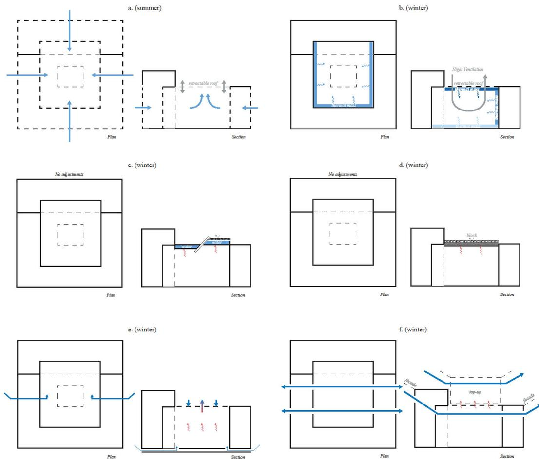
Figure 7. Implementation of passive cooling strategies in typical performance building typology. Direct connection theatre and ambient air (a), Thermal mass with night ventilation (b), Indirect evaporative cooling through the roof (c), Radiative cooling through the roof (d), Buoyancy effect (e), Wind-driven cross ventilation (f).
