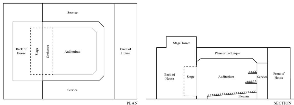
Figure 2. Typical layout of a performance building.
