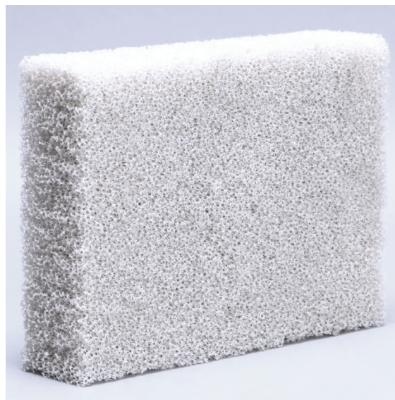
Figure 21. A Sawbones® 15 PCF cellular foam block with a thickness of 40mm
