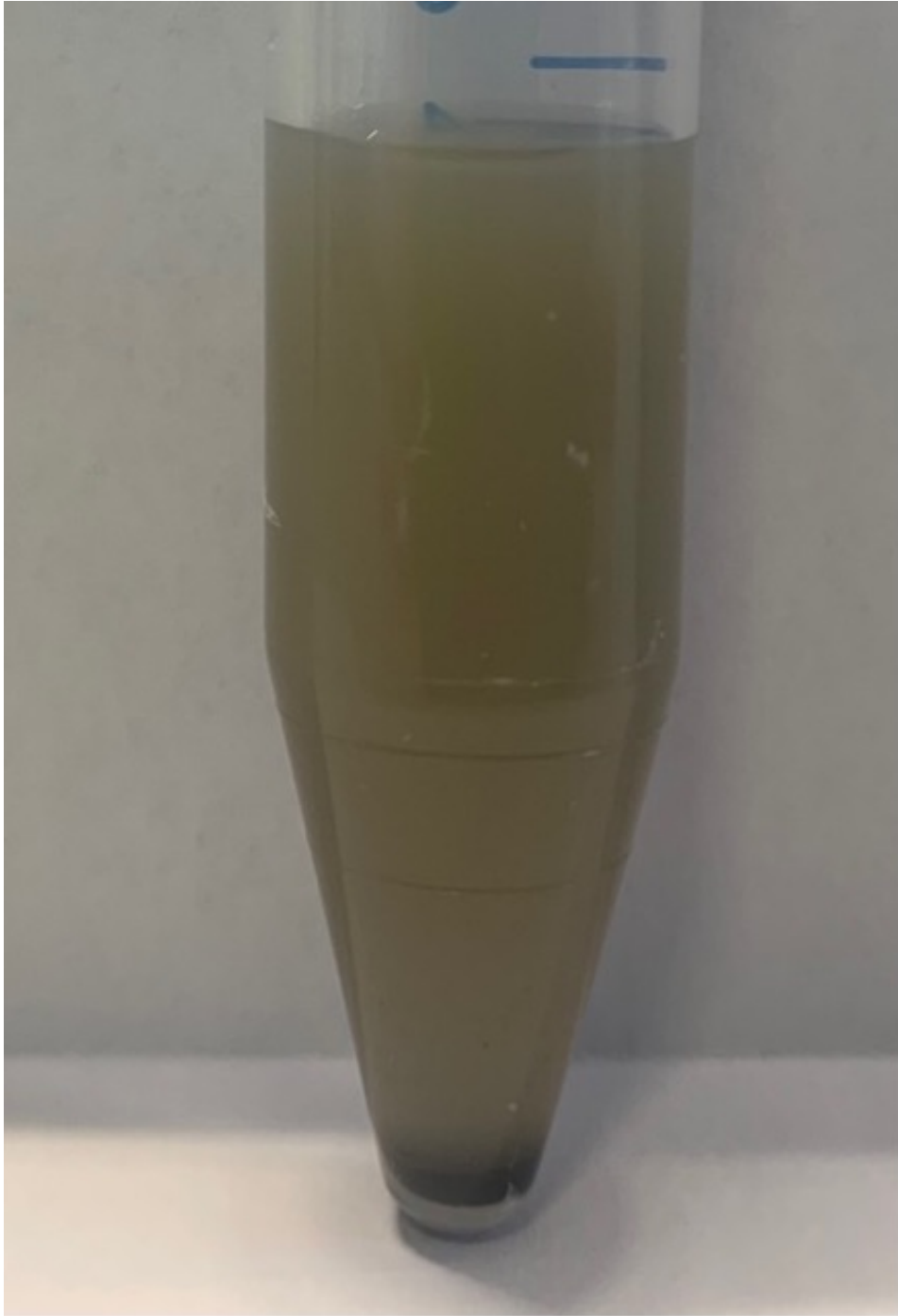
Figure B.2: Partly sedimented loaded SU-8 2007 (0.25 wt.%), one day after preparation.
