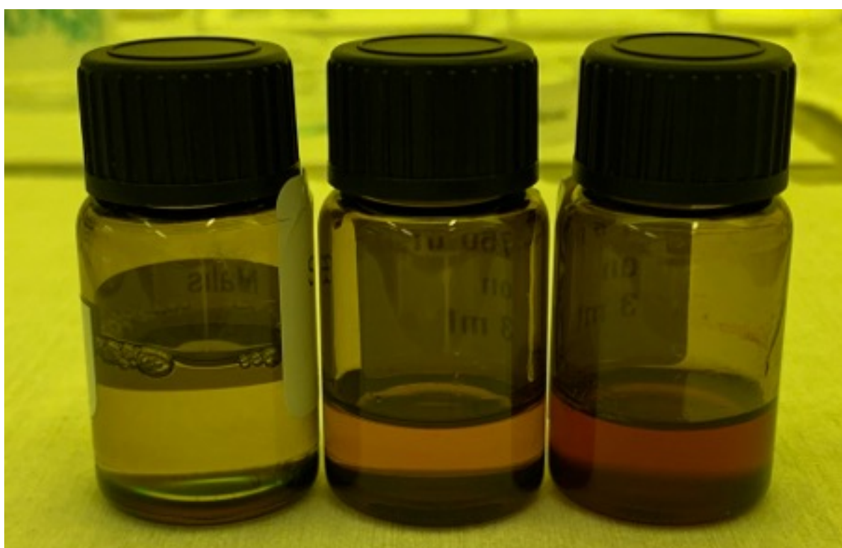
Figure D.1: Optical image of SU-8 2075, ND loaded SU-8 2075 with 0.5 wt.% and 1 wt.% from left to right, respectively.
