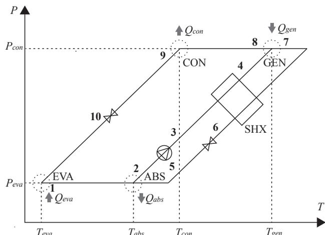
Fig. 2. The single-effect AHP cycle on a  $\ln P - (-1/T)$  diagram.
