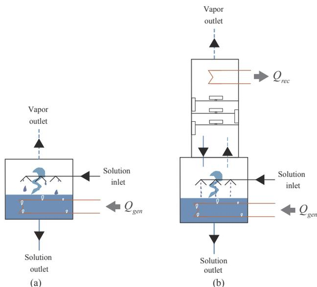
Fig. 3. Two constructions of the generator. (a) The generator for working pairs using absorbents with a negligible vapor pressure at operating temperature, say  $NH_3/ILs$  in this study. (b) The generator with purification section above it (distillation column and rectifier) for working pairs using absorbents with a non-negligible vapor pressure at operating temperature, say  $NH_3/H_2O$  in this study.
