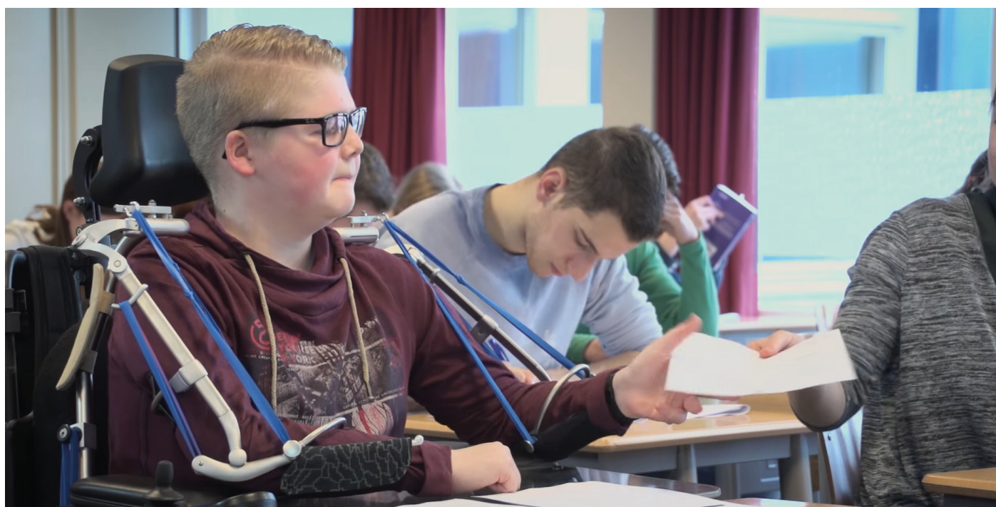
Fig. 3 The A-gear (Flextension): first prototype of a passive exoskeleton for Duchenne boys
