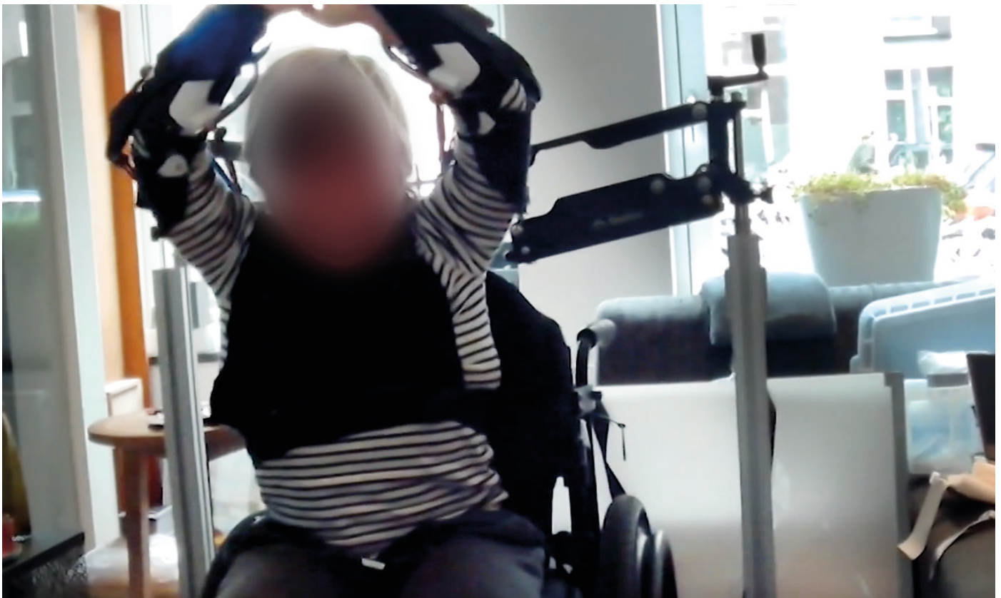
Fig. 7 The passive exoskeleton gives Duchenne boys the ability to move their arms how they want to
