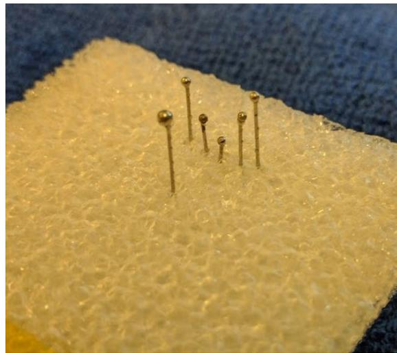
Figure III.2.2: The phantom used in setup 2. It consists of tiny needles with a small ball at the top that has a diameter in the order of 1 mm.
