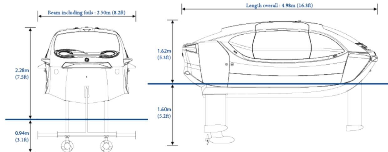
Figure 2: Dimensions of the seaBubble for seven passengers (SeaBubbles, n.d., b)
