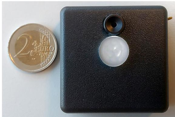
Figure 1.2: Our proposed hardware platform that houses a thermopile sensor and a PIR sensor.
