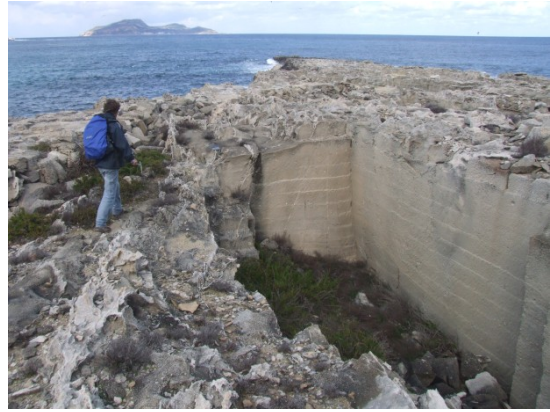
(b) Punta San Vituzzo with massive calcarenite and Levanzo in the background. Note the horizontal marks made by the quarrying equipment.
