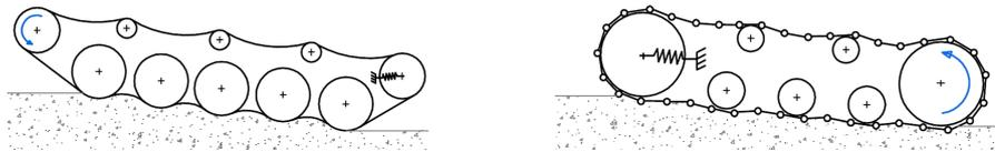
Figure 2.18: Flexible type track belt (left) and rigid type track belt (right), image from [Daanen, 2017].
