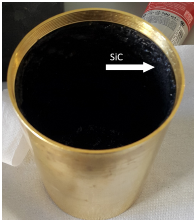
Figure 3.16: A cylindrical copper shield with a gold coating on the surface. Inside of the shield is coated by SiC, which serves as an absorber for infrared radiation.
