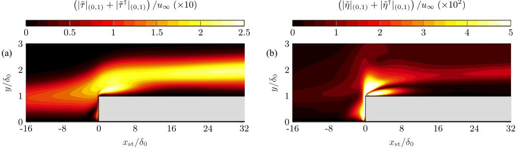
FIG. 4. Amplitude function of fundamental (a) streamwise,  $|\tilde{\tau}|_{(0,1)}$ , and (b) cross-stream,  $|\tilde{\eta}|_{(0,1)}$ , velocity perturbations.
