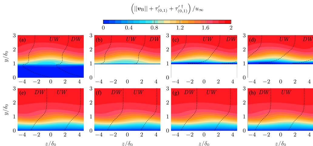
FIG. 8. Steady total streamwise flow (color contour), in  $y$ - $z$  planes for the step (top) and reference no-step (bottom) cases at  $-0.02$  [(a), (e)],  $0.04$  [(b), (f)],  $0.52$  [(c), (g)],  $1$  [(d), (h)]. Dashed lines segregate cross-stream-perturbation upwash (UW) and downwash (DW); see Fig. 7 for reference.
