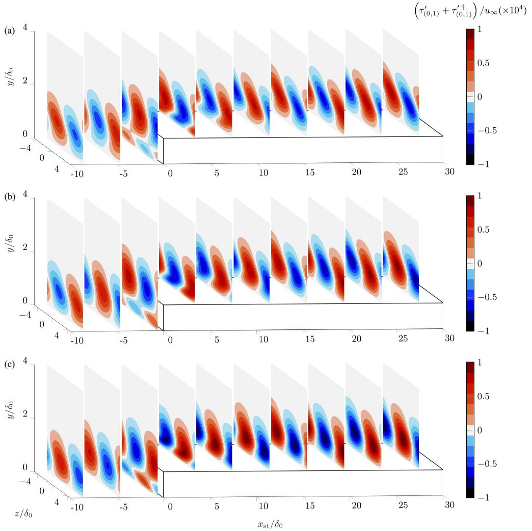
FIG. 16. Organization of the streamwise-velocity perturbation for  $\beta = \beta_0$  in cases Test A (a), B (b), and C (c) of Table I.
