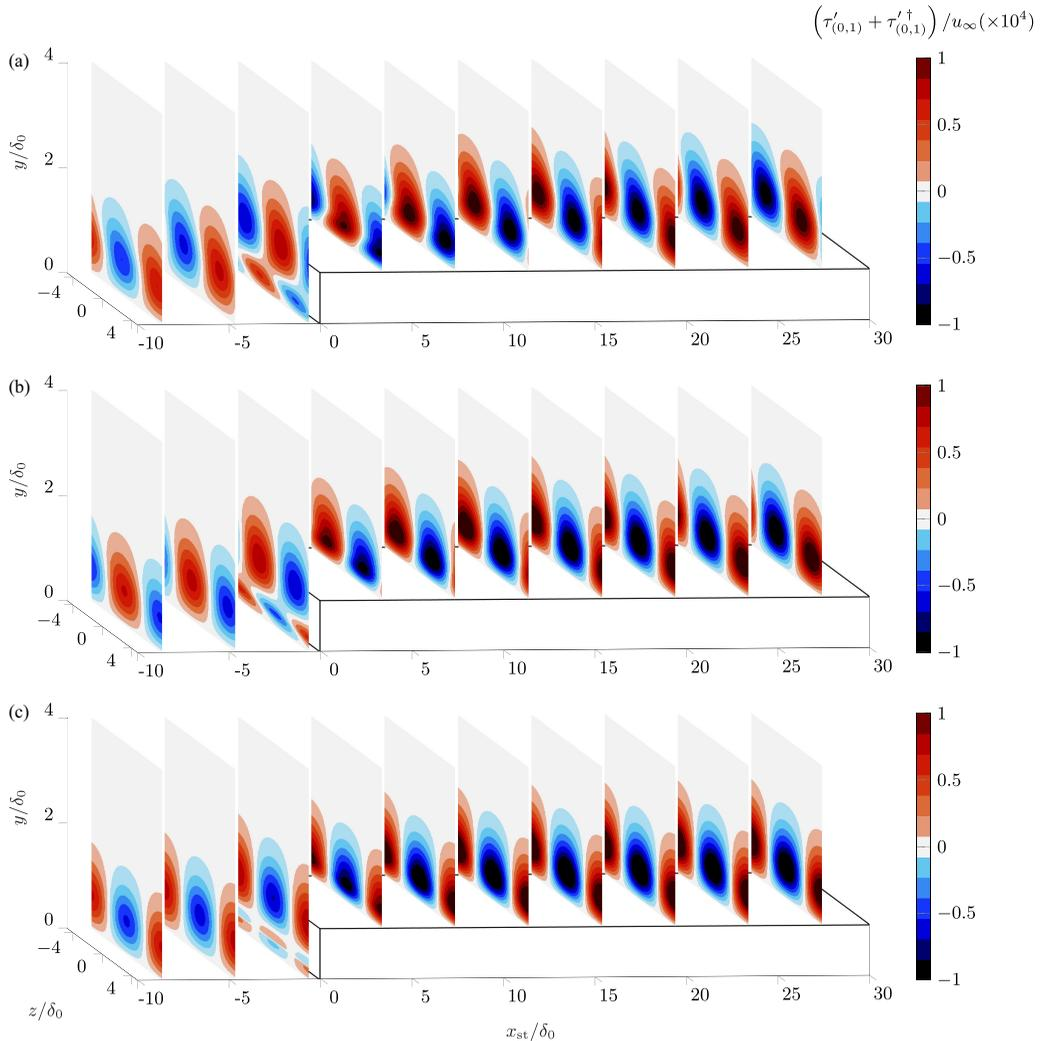
FIG. 17. Organization of the streamwise-velocity perturbation for  $\beta = \beta_0$  in cases Test D (a), E (b), and F (c) of Table I.
