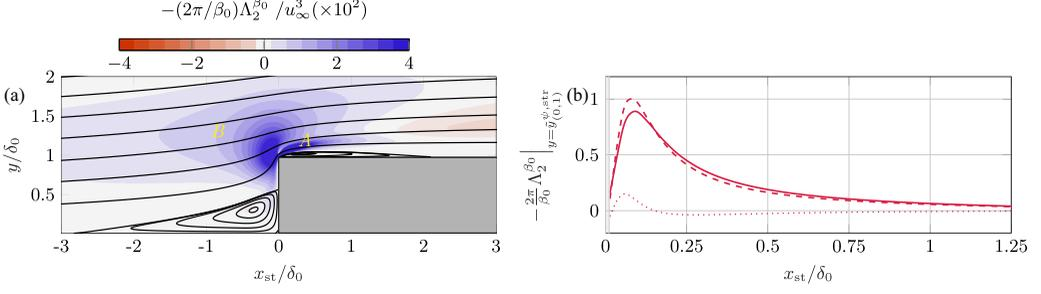
FIG. 6. Spatial evolution of  $(-2\pi/\beta_0)\Lambda_2^{\beta_0}$  [Eq. (16)] with cross-sectional streamlines of the base flow (a) and chordwise evolution of individual terms of Eq. (16) at the wall-normal location of the core of the streaks (b):  $(-2\pi/\beta_0)\kappa_2^{\beta_0}$  [solid, see Eq. (20)], remainder (dotted), global term  $(-2\pi/\beta_0)\Lambda_2^{\beta_0}$  (dashed). All curves are normalized relative to maximum  $\Lambda_2^{\beta_0}$ .
