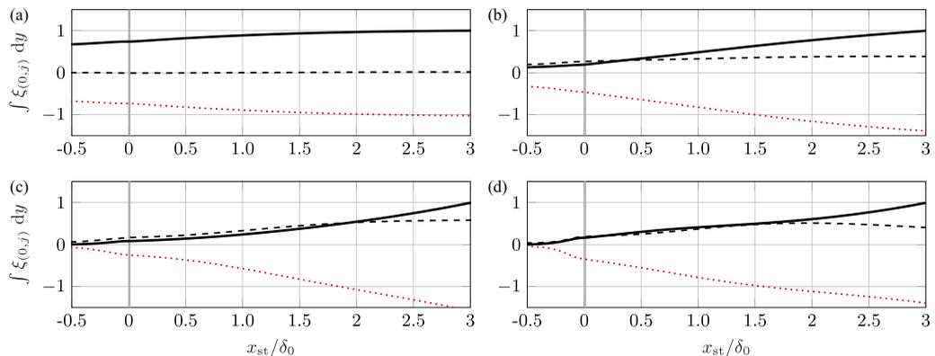
FIG. 12. Chordwise evolution of integral budget terms of the energy-balance equations of the spanwise-harmonic perturbation modes:  $\xi$  identifies linear production (solid black), the work of nonlinear interactions (dashed black), and the remainder of linear mechanisms (dotted red) for the stationary perturbation modes  $j = 1$  (a), 2 (b), 3 (c), and 4 (d). All curves are normalized relative to the maximum of linear production in each subplot.
