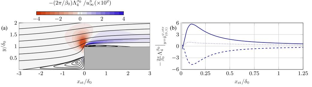
FIG. 9. Spatial evolution of  $(-2\pi/\beta_0)\Lambda_4^{\beta_0}$  [Eq. (21)] with cross-sectional streamlines of the base flow (a) and chordwise evolution of individual terms of Eq. (21) at the wall-normal location of the core of the streaks (b):  $(-2\pi/\beta_0)\chi_4^{\beta_0}$  (solid), sum of remainder (dashed), global term  $(-2\pi/\beta_0)\Lambda_4^{\beta_0}$  (dotted). All curves are normalized relative to  $\max(\Lambda_4^{\beta_0})$ .
