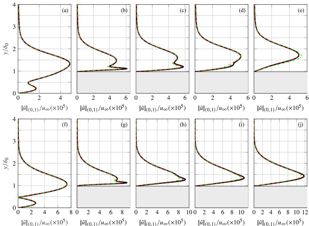
FIG. 1. Profiles along  $y$  of the amplitude function  $|\tilde{u}|_{(0,1)}$  at the step from DNS (solid black), AHLNS (dash-dotted green), and DeHNSSo (dashed red) at  $x_{st}/\delta_0 = -0.5$  [(a), (f)],  $0.5$  [(b), (g)],  $2.5$  [(c), (h)],  $5$  [(d), (i)],  $10$  [(e), (j)]. Top row illustrates case  $\max(|w_\infty/u_\infty|)$  and bottom row illustrates case  $w_\infty/u_\infty = 0$ .
