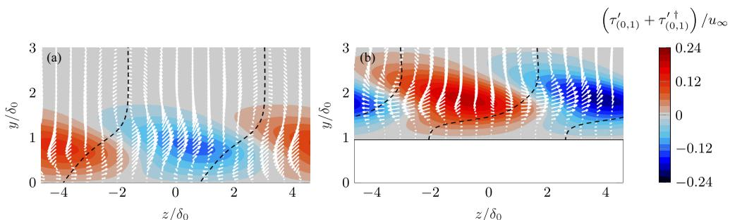
FIG. 15. Organization of streamwise-velocity (color contour) and in-plane cross-stream-velocity (white arrows) perturbations in  $y$ - $z$  planes upstream,  $x_{st}/\delta_0 = -10$ (a), and downstream,  $x_{st}/\delta_0 = 20$ (b), of the step in case Baseline of Table I. Dashed black lines segregate cross-stream-perturbation upwash and downwash.
