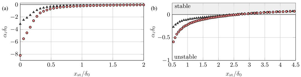
FIG. 10. Spatial growth rates of the total,  $|\tilde{\psi}|_{(0,1)}$  (triangles), and streamwise,  $|\tilde{\tau}|_{(0,1)}$  (circles), perturbations at the wall-normal location of streaks,  $y = \tilde{y}_{(0,1)}^{w, \text{str}}$ , in the ranges  $0 \leq x_{\text{st}}/\delta_0 \leq 2$  (a) and  $0.5 \leq x_{\text{st}}/\delta_0 \leq 4.5$  (b).
