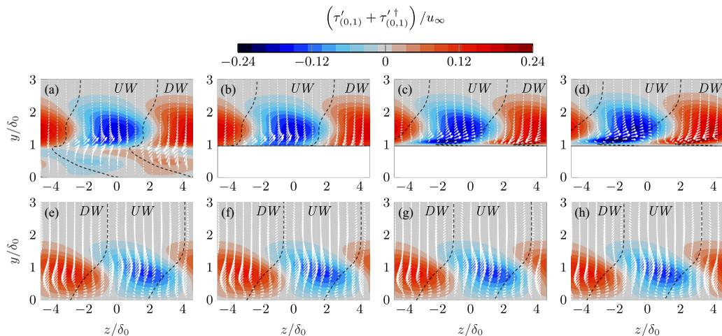
FIG. 7. Streamwise-velocity perturbation (color contour) in  $y$ - $z$  planes for the step (top) and reference no-step (bottom) cases at  $-0.02$  [(a), (e)],  $0.04$  [(b), (f)],  $0.52$  [(c), (g)],  $1$  [(d), (h)]. In-plane organization of the cross-stream-velocity perturbation (white arrows). Dashed lines segregate cross-stream-perturbation upwash (UW) and downwash (DW).
