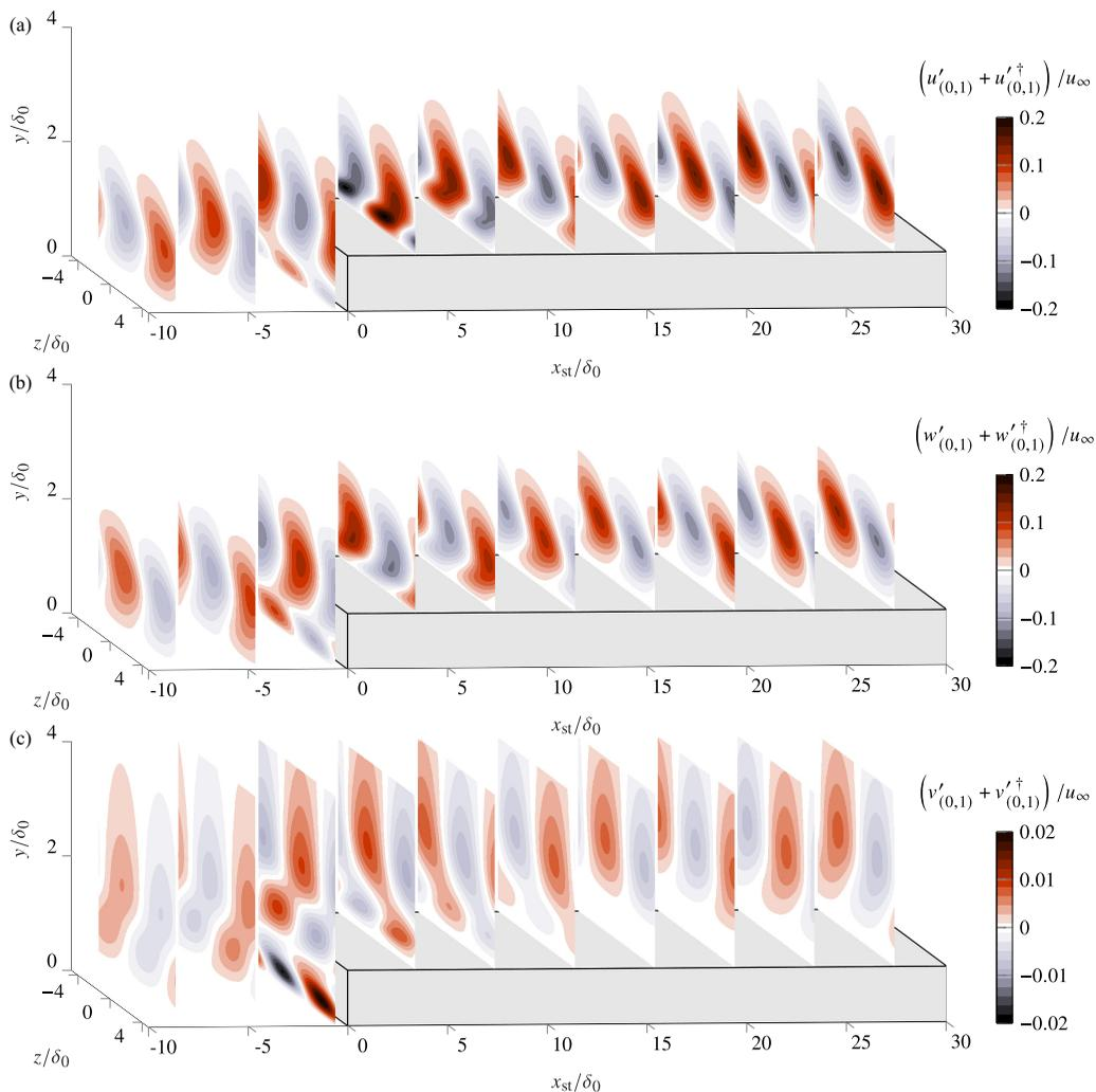
FIG. 2. Organization of the chordwise (a), spanwise (b), and wall-normal (c) fundamental velocity-perturbation fields ( $\beta = \beta_0$ ). Note the different scale in plot (c).
