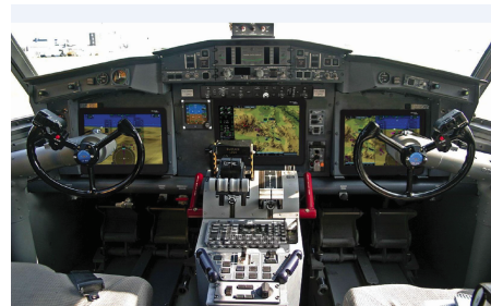
(b) CL-415 improved future avionics panel
