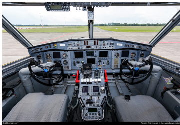
(a) CL-415 Old avionics panel
