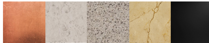
Aging Copper Thresholds Italian White Monumental walls Italian Terrazzo Hallway flooring Recycled Crushed Italian Beige Hallways floor/walls Opaque glass Interior smart glass
