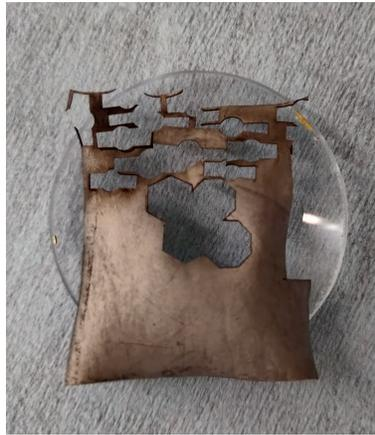
Figure 21: IPMC sample ( $12 \times 12 \text{ cm}^2$ ) used for density measurement.
