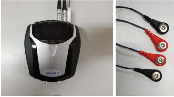
Fig. 2. Mangold-10 wireless Bluetooth multi-channel physiology system made in Germany.
