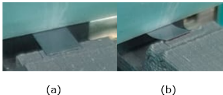
Figure 6.4: (a) shows a custom made force indenter making contact with the backside of die (silicon) (b) thin die bending under applied load. ultra-thin silicon dies shows extraordinary flexibility
