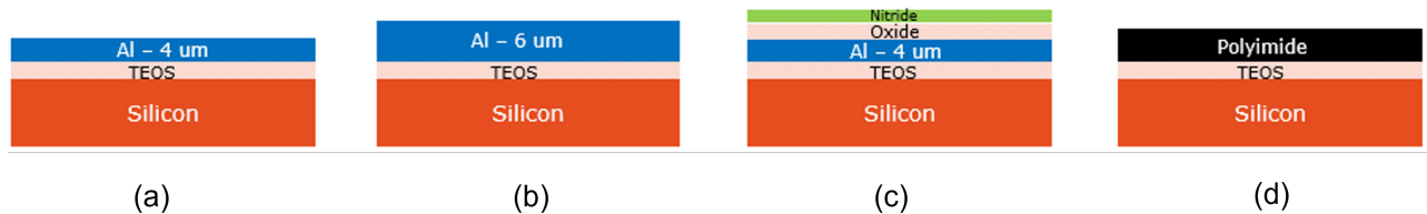
Figure 3.16: The figure shows different die cross-sections with various semiconductor process layers. Die cross-section are namely (a) Si + 4 \mu\text{m} Al die; (b) Si + 6 \mu\text{m} Al die; (c) Si + 4 \mu\text{m} Al + passivation layers; (d) Si + 5 \mu\text{m} PI
