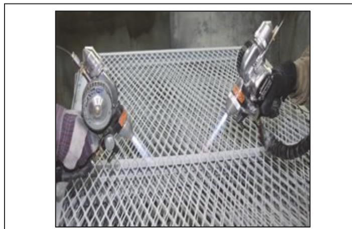
Figure 2-51 – Thermally Sprayed Metal Coating process, using a wire-source and a hand sprayer (Avant Guards Coatings)
