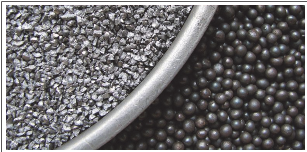
Figure 2-55 - Grit (left) and shot (right) particles used for abrasive blast cleaning (Mogilev Metallurgical Works)
