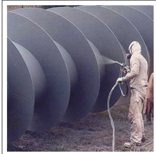
Figure 2-54 - Application of alkali zinc silicate coating (Ashok Paint Agencies)
