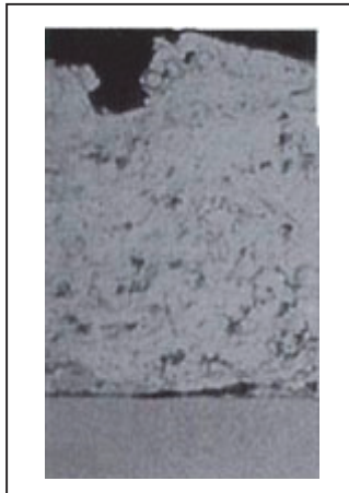
Figure 2-52 - Cross section of a thermally metal sprayed coating (Lindsley, 2016)
