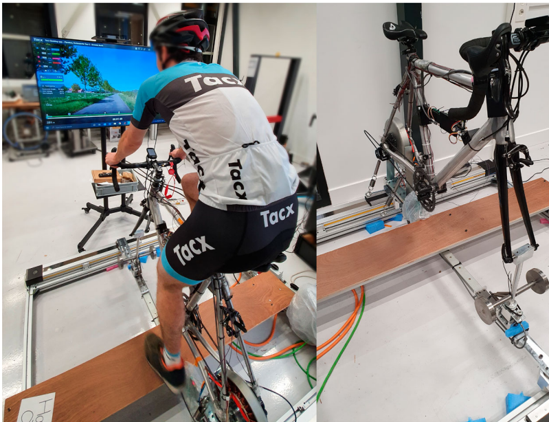
Figure 3. Bicycle simulator mechanical setup. The visualisation screen, the used bicycle frame and the electromechanical system are visible. Springs at the rear of the bicycle keep the bicycle in its upright position, and a mass-spring combination at the front of the bicycle provides steering resistance to the user.
