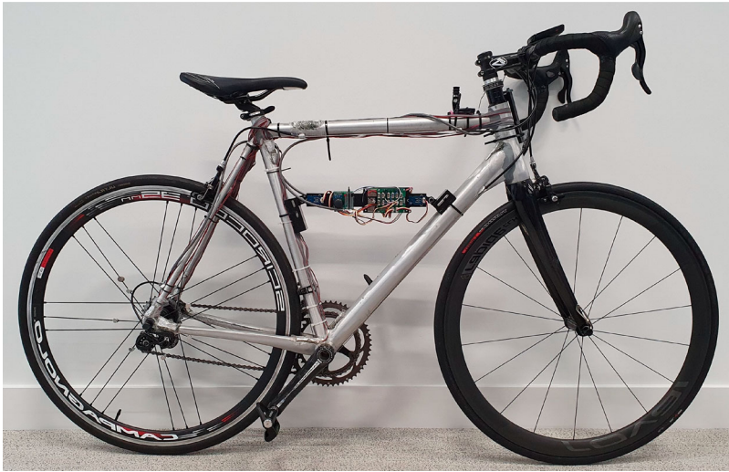
Figure 5. Custom racing bicycle used for outdoor experiments. Includes the kinematics measurement board in the centre of the frame. Magnets in the rear wheel are used for velocity measurements. Saddle is adjustable for participants.
