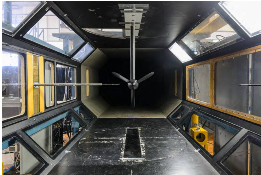
Fig. 3 Propeller setup for regenerative-propeller experiment installed in Delft University of Technology's Low-Turbulence Tunnel.
