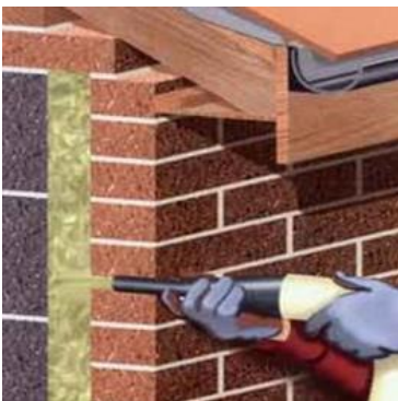
Fig. 3. Placement method of cavity insulation.
