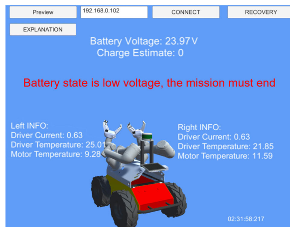
FIGURE 12. Low battery error message displayed in the DT alongside color-coded alert system in red on the mobile base indicating the health status of the robotic platform.
