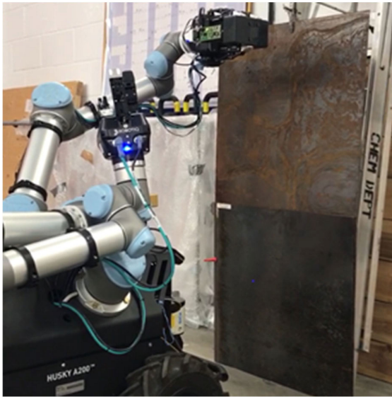
FIGURE 18. Husky A200 with a pair of UR5 manipulator arms integrated with the FMCW inspection tool during a corrosion inspection; the top sheet is lightly corroded steel and the lower sheet is non corroded and polished.
