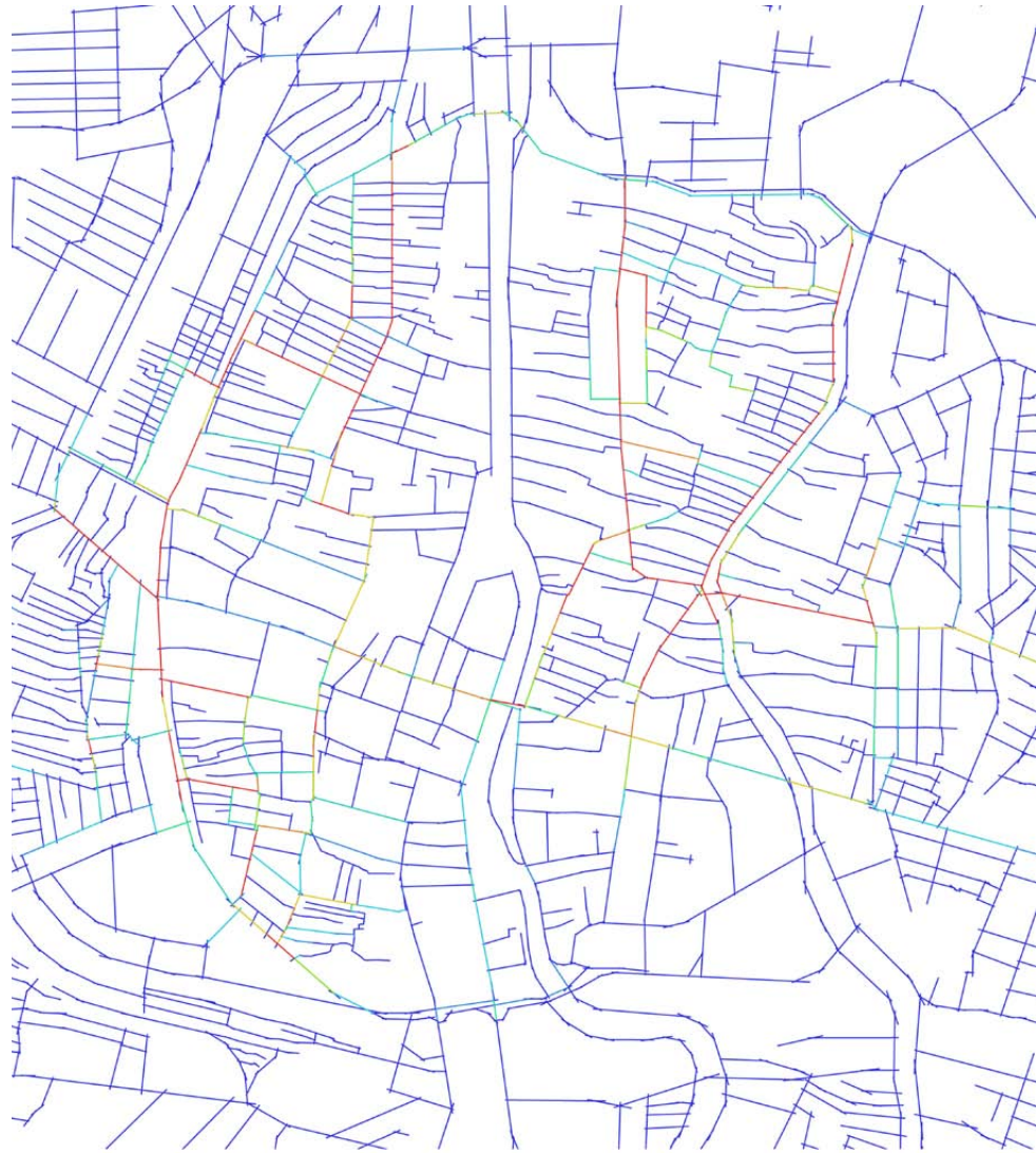
Figure 6.2. Space syntax analysis : Topological Metric R10 on current condition of Old Town Surabaya
