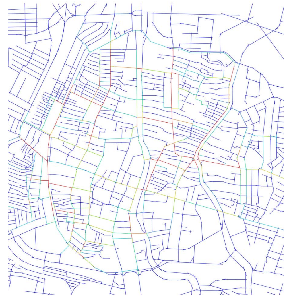
Figure 6.4. Space syntax analysis : Topological Metric R10 on future condition of Old Town Surabaya (Author's Plan)
