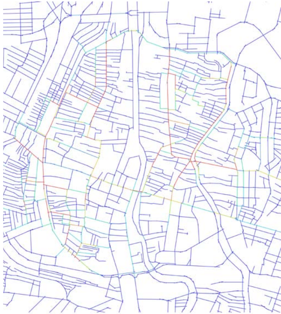
Figure 3.41. Space syntax analysis : Topological Metric R10 on current condition of Old Town Surabaya
