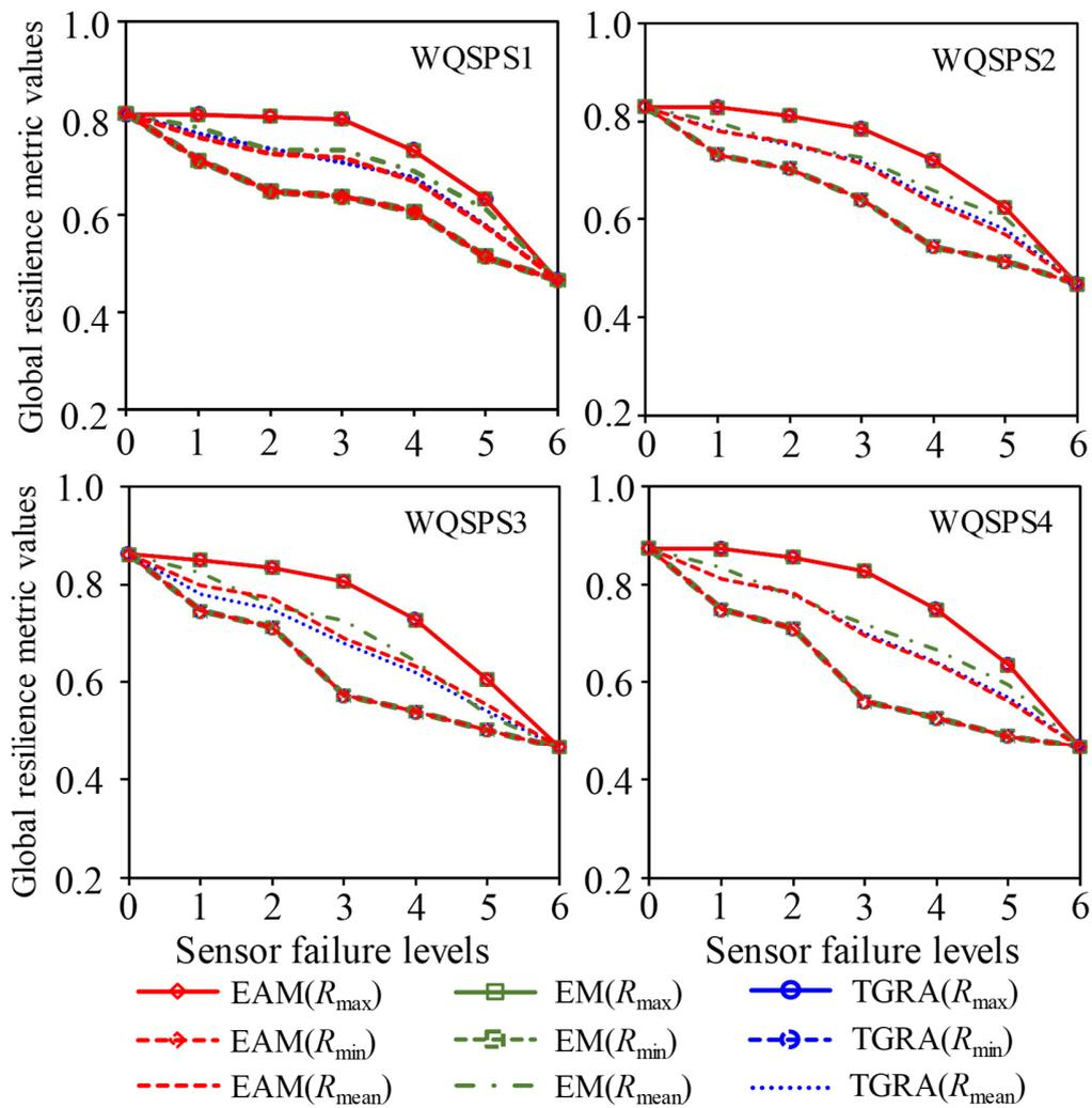
417 **Fig. 8. Global resilience metric values of different failure levels applied to the four different**
