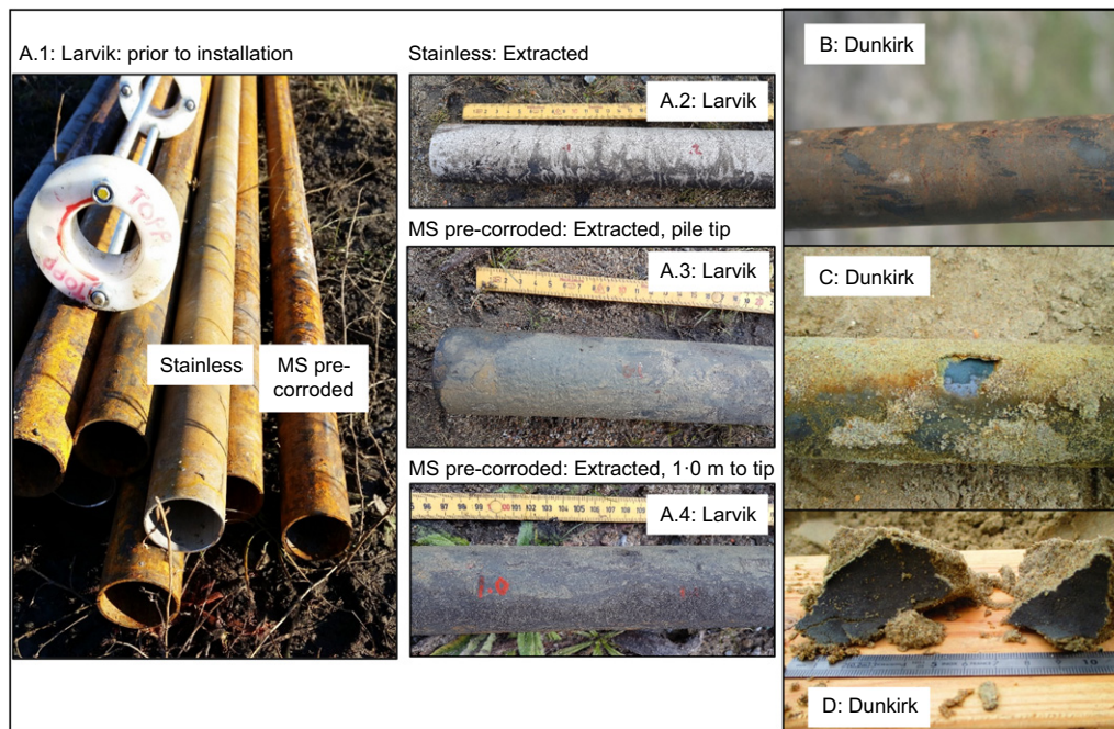
Fig. 8. (Label A.1) Larvik pre-corroded MS and stainless steel piles, before use November 2015; (labels A.2–A.4) Larvik extracted piles, pulled out October 2017; (label B) Dunkirk pre-corroded pile before use; (label C) Dunkirk fresh MS extracted pile, dug out; and (label D) Dunkirk oxidised sand taken from face of a MS pile after extraction
