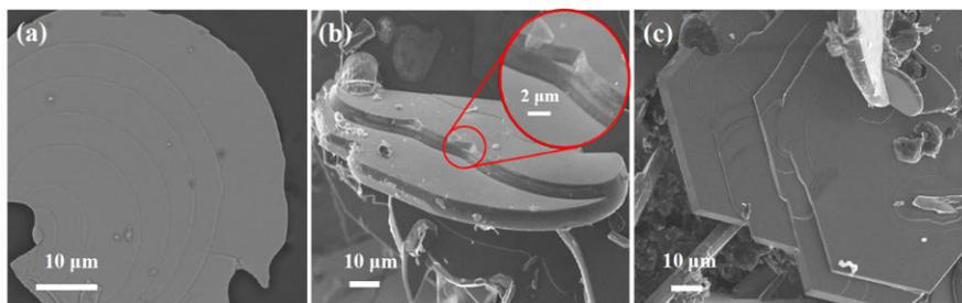
**Fig. 4** SEM images of synthesized  $\text{Al}_4\text{SiC}_4$  grains with different morphologies. (a) Grain with shallow smooth edges and striations; (b) grain with thick smooth edges and striations; (c) the well-developed grain with straight edges and sharp corners.
