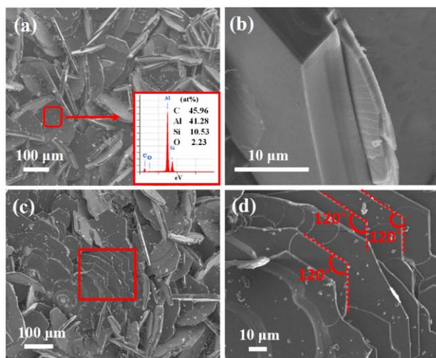
Fig. 2 SEM images of the synthesized  $Al_4SiC_4$  powders by carbothermic reduction. (a) General morphology of synthesized  $Al_4SiC_4$  powders, the inset: EDS analysis of the grain in the rectangle in (a); (b) thickness of the grains; (c) and (d) detailed stacking layer of  $Al_4SiC_4$  grains with hexagonal plate-like feature; (d) enlarged SEM image of the red rectangle in (c).
