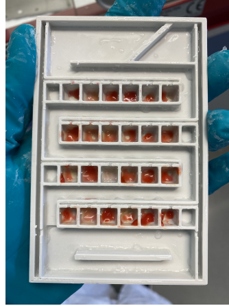
Figure 2.14: The cartridge after the saturation in ethanol. The red colorant is the marker for the next step experiment.
