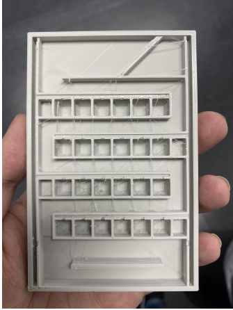
Figure 2.13: The fibers on the surface of the cartridges. The fibers are mainly found around perpendicular structures.
