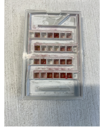
Figure 2.15: The white residue concentrates on the surface of the cartridge after drying, making the cartridge unusable.
