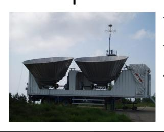
TARA (S-band RADAR) measures the vertical Doppler verlocities at Cabauw.
