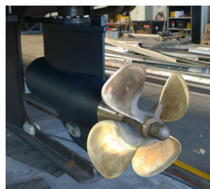
Figure 3.7: Schematic of POD drive [11]
