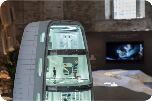
Figure 3 Moon village design for the 2021 Venice Architecture Biennale by SOM (Ghinitoiu 2021). It features a spiral staircase with a riser same as on Earth, while the gravity on the Moon is significantly lower.
