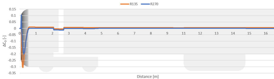
Figure 4.2: Difference in drag development for the basic model with different leading edge radii, R540 is used as baseline
