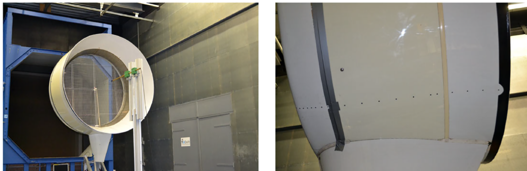
FIGURE 2 Pictures showing the experimental set-up with hot-wire anemometer placed on the traversing system (left) and pressure taps along the duct surface (right) [Colour figure can be viewed at wileyonlinelibrary.com ]
