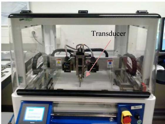
**Figure 2:** Scanning Acoustic Microscope (SAM), available in TNO Eindhoven, The Netherlands.
