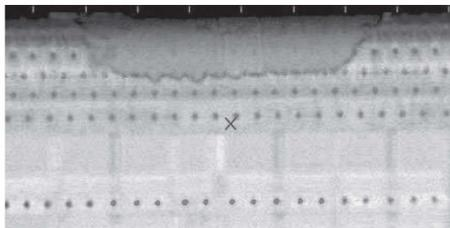
**Figure 5:** SAM image of a flip chip with cracking in the low k dielectric layers [2]
