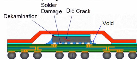
**Figure 1:** Schematic of a package with location of some failures
