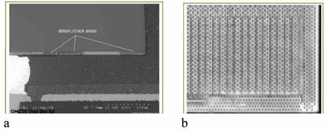
**Figure 7a)** shows ILD cracks and Xb) how it looks like under SAM [7]
