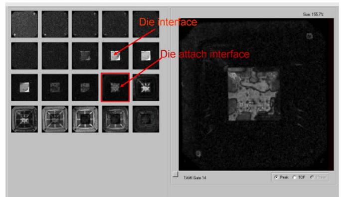
**Figure 4:** Tomographic Acoustic Micro Imaging (TAMI) mode in SAM [3]
