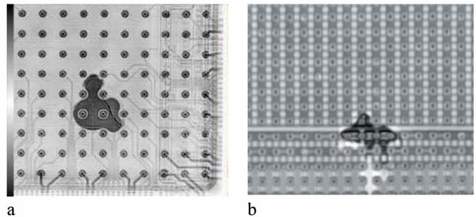
**Figure 8:** Two underfill voids observed by SAM. Void above the underfill is white, while the other one below the underfill is black [8,9]
