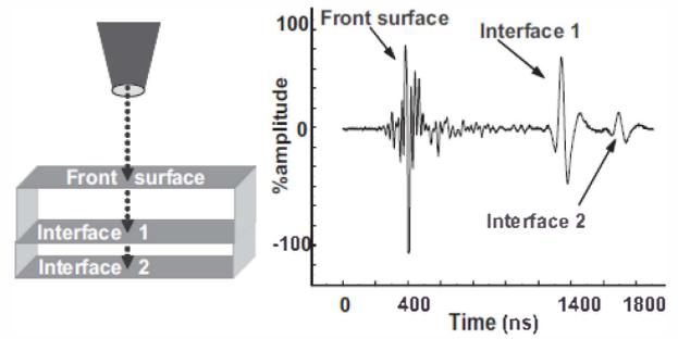
**Figure 3:** A-scan over the thickness of the sample [2].
