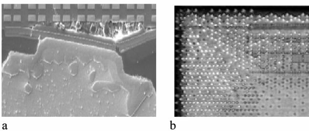
**Figure 6a)** shows fracture at the interface of solder ball and the dielectric and 6b) is how it looks like under SAM [6]
